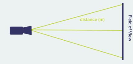
It is important to consider both the mounting height and viewing angle of the camera. If the camera is placed too high, or the horizontal/vertical angle is too big, the recognition accuracy may be reduced.
