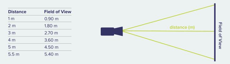
It is important to consider both the mounting height and viewing angle of the camera. If the camera is placed too high, or the horizontal/vertical angle is too big, the recognition accuracy may be reduced.
