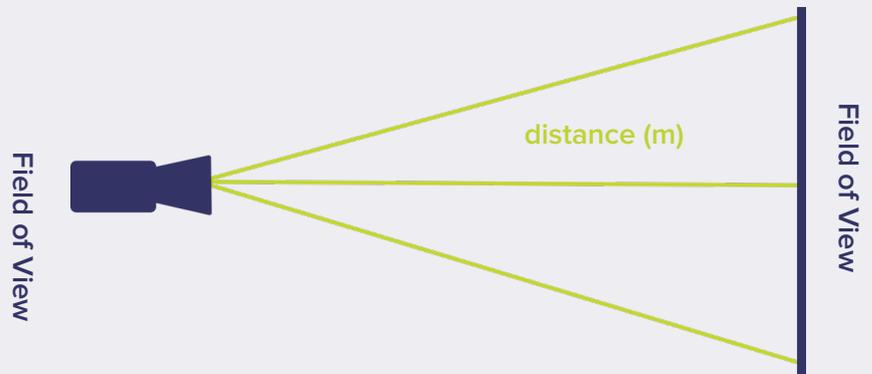
It is important to consider both the mounting height and viewing angle of the camera. If the camera is placed too high, or the horizontal/vertical angle is too big, the recognition accuracy may be reduced.
