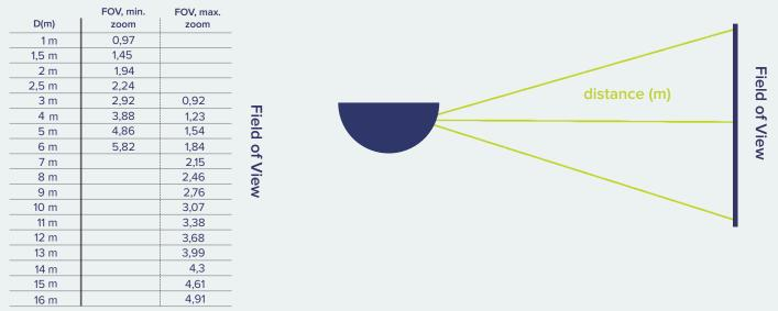
It is important to consider both the mounting height and viewing angle of the camera. If the camera is placed too high, or the horizontal/vertical angle is too big, the recognition accuracy may be reduced.
