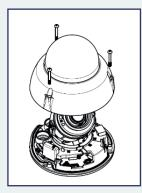
**2.** Loosen the Philips head screws, adjust the camera angle, then retighten the screws. Finally, attach the top cover.
